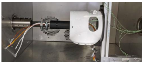
Figure 5: Harness Thermal Chamber twist test configuration.
